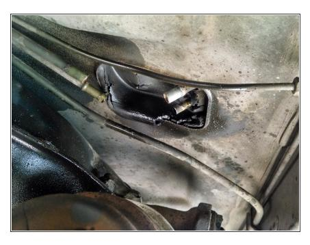
With all four clamps loosened, pull both lines off. You can see here what the metal fuel lines look like with the lines removed.
