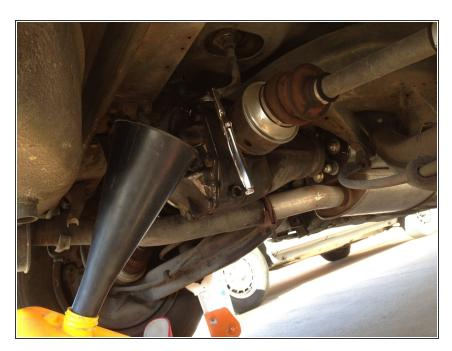
Position your catch container near the main fuel feed line. Using a container that you can insert a long funnel in will be helpful. It should be large enough to hold the amount of fuel you estimate to be in the tank. Or, you should have multiple containers on hand.
