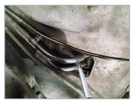
Loosen all four of the hose clamps on both fuel lines using a Phillips or flathead screwdriver as needed.
