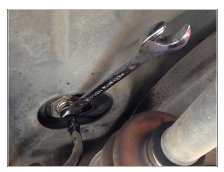
Once the tank is fully drained you will need to use a 19mm wrench to remove the main fuel feed line from the tank.
