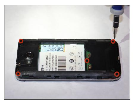
Remove the five 4mm Philips #00 screws, circled in red, holding the the back down.
