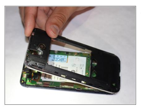
Remove the back piece, exposing the motherboard.
