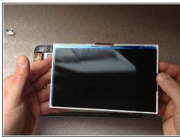
Lift the display up and remove it.
