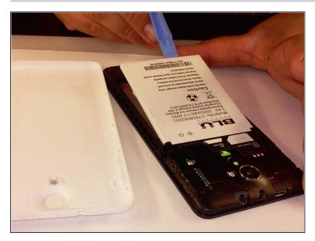
• Remove the battery from the phone with the plastic opening tool, or your fingers.
