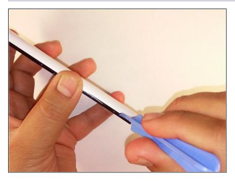
• Remove the back cover of the phone with the plastic opening tool, or your fingers.
