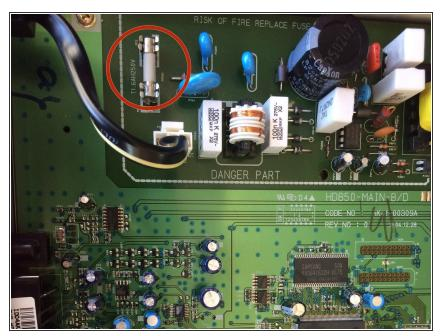
• Locate the power fuse on the bottom left of the circuit board
