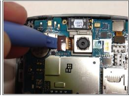
Repeat the same process for the other 3 ribbon cables connected to the motherboard
