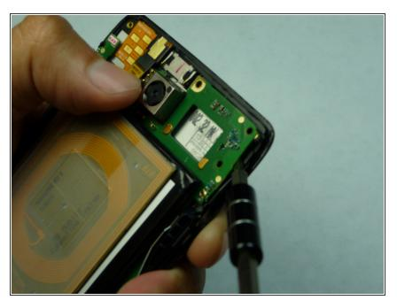
Start by lifting the motherboard using a prying plastic tool
