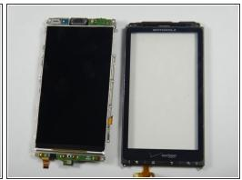
Lift the screen off of the device
