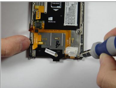
Remove the 4 screws using a T-3 torques.. These screws are 2.40 mm in length.
