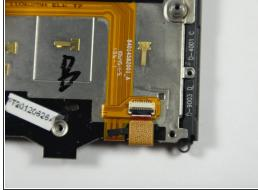
Using tweezers, remove the white tape to reveal the connector
