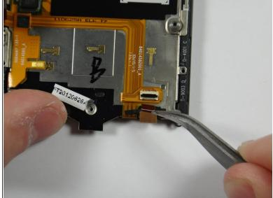
Using tweezers, remove cable from the connector
