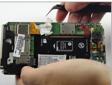
Using tweezers, removed the white electrical tape on the motherboard.
