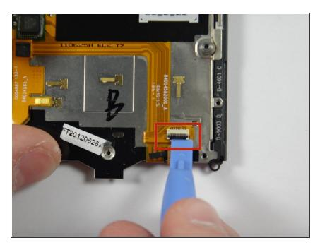
Using the plastic opening tool, lift the jawbone connector.
