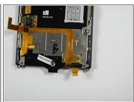
Using a plastic opening tool, lift the connector from the device
