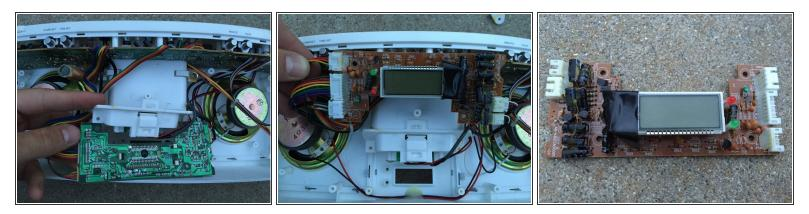
• Removing the LCD Panel and motherboard.
