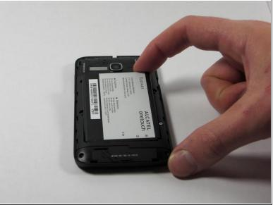
Place finger in the tab on the top right corner of the battery indicated by a black arrow. With slight pressure, push battery down and out of the slot until the battery is removed
