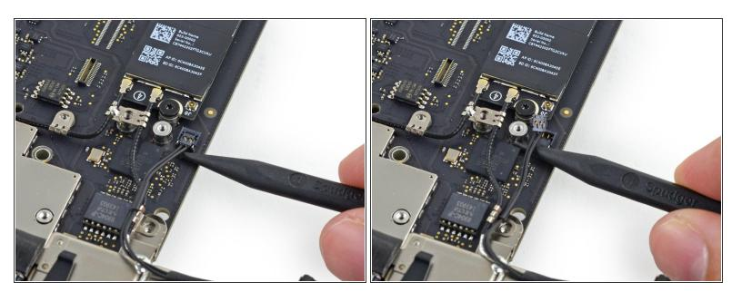
Use the point of a spudger to lift the power switch cable connector straight up out of its socket on the logic board.
