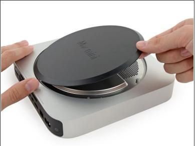
Lift and remove the bottom cover.
