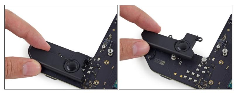
♠ Do not attempt to remove the speaker entirely as it is still attached to the logic board.
