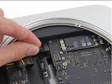
Pull the DC-In cable connector straight out of its socket on the logic board.
