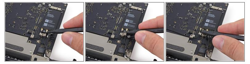
• Use the point of a spudger to lift the antenna connectors up off of their sockets on the AirPort card.
