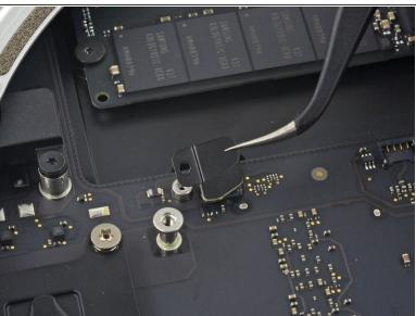
Remove the SATA cable connector bracket.
