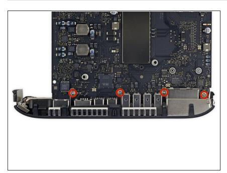
Remove the four 2.7 mm T6 Torx screws holding the I/O bezel to the logic board.
