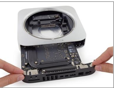
Carefully slide the logic board assembly out of the Mac mini, minding any cables that may get caught.
