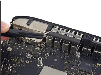
Remove the foam bumper from between the I/O bezel and USB ports.
