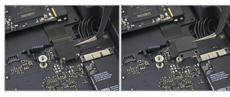
Remove the PCIe SSD cable bracket.
