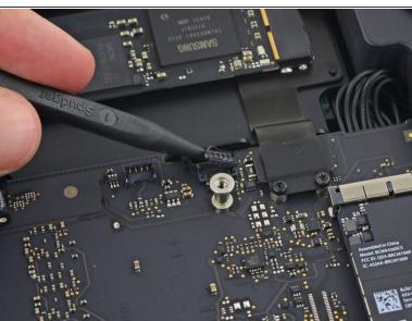
Use the tip of a spudger to disconnect the IR sensor cable connector by prying it straight up from its socket.
