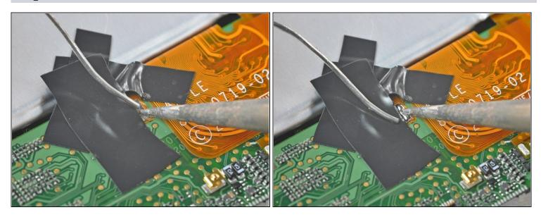
Place your battery in the rear panel, with the cable side down, and use two small strips
