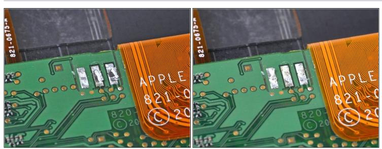
• Next, use the tip of a soldering iron to flatten out the solder on the logic board solder pads. The pictures show a 'before' and 'after' shot.
