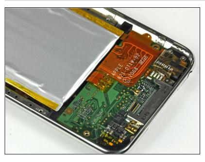
Don't forget to reapply the piece of tape over the solder pads to prevent any shorts.
