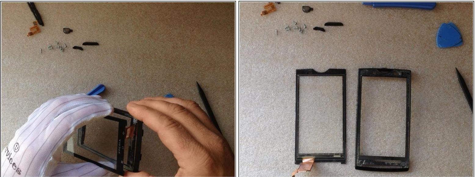
**i** When you are installing the new Touchscreen you must use an adhesive tape.
