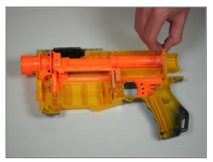
• Lift the plunger guide straight up out of the gun.
