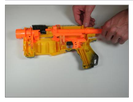
Pull the remaining half of the plunger out the back of the gun.
