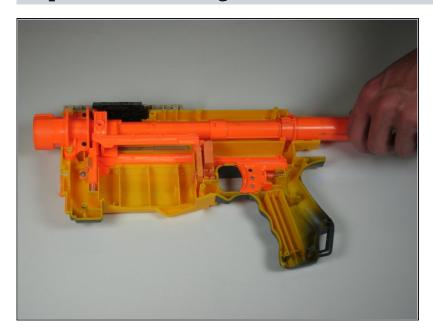
Pull the plunger out the back of the gun off of the inner piece.
