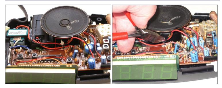
• Using the wire cutters, carefully cut the plastic wire tie.
