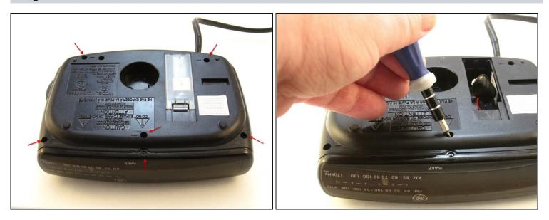
• Using a Phillips #00 Screwdriver, unscrew the six 12mm screws from around the bottom of the clock radio.
