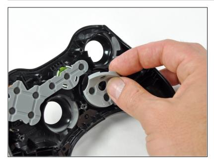
Remove the rubber pad from the back of the D-pad.
