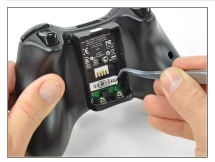
Use a pair of <u>tweezers</u> to peel the barcode sticker from the battery compartment.
