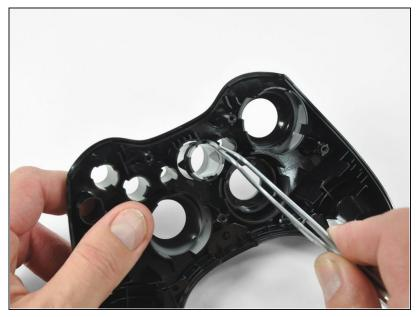
Using a pair of tweezers, remove the LED ring from the front panel.
