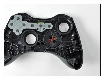
Remove the two 7.0 mm silver Phillips screws from the back of the D-pad.
