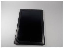
• wedge the plastic opening piece underneath the bottom left hand corner of the front frame. Pry the frame off of the Nook.
