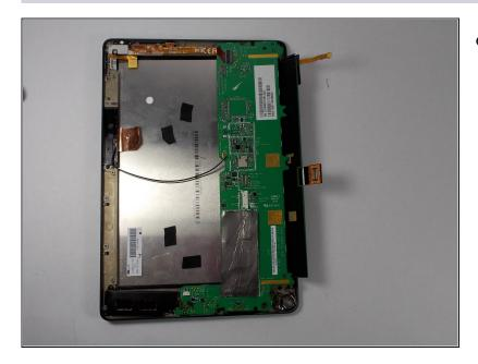
• flip center chassis so that the back of the screen is facing you, and the hole is positioned in the bottom right corner.
