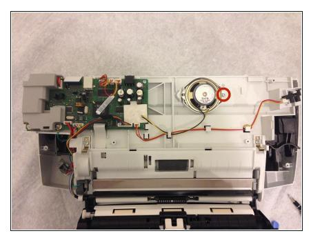
Using your Torx t10 screwdriver, remove the screw located on the right side of the speaker as shown in the figure on the left. The screw is 13mm in length.
