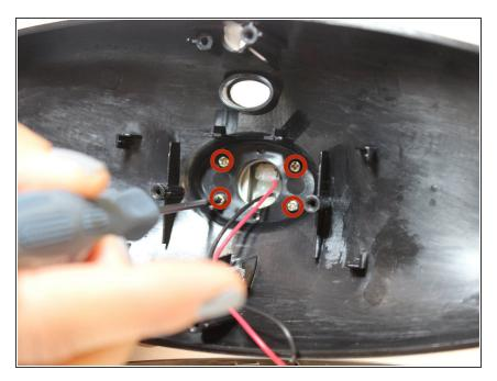
• Use the Philips #00 screwdriver to remove the four 6mm screws from the base cover.
