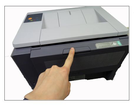
Open back of printer by pushing down handle.
