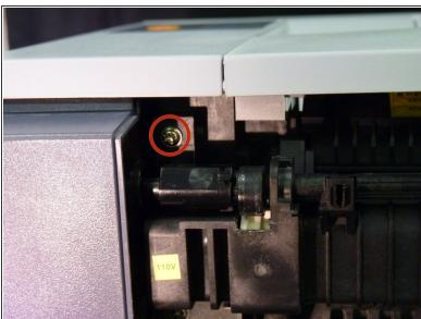
Remove the four screws that attach the fuser unit to the printer.
