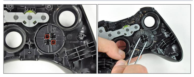
i The D-pad is secured to its backing by two diagonal clips, shown in red.
