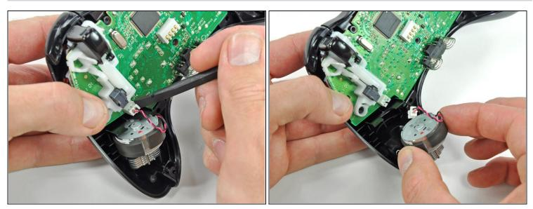
• Remove the vibration motor from the other side of the controller using the same method previously described.
