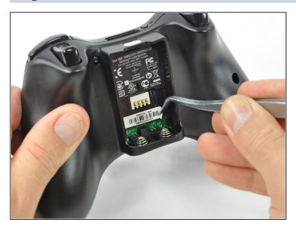
• Use a pair of <u>tweezers</u> to peel the barcode sticker from the battery compartment.
