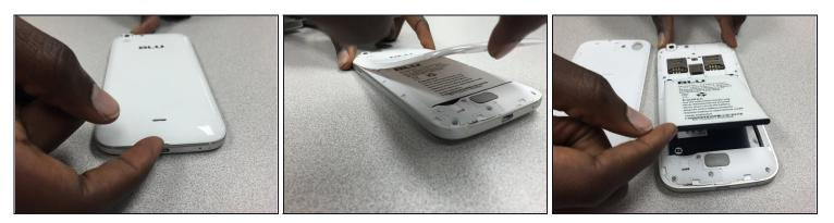
• Remove the cover by lifting the notch towards the bottom of the phone. Use your fingernail to lift it up.
