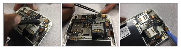
• Using a spudger, peel up on the mesh tape then use your <u>tweezers</u> to peel the rest of it up.
