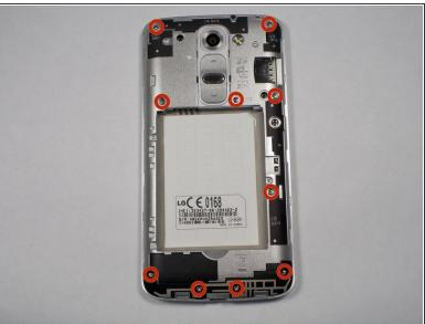
Locate 10 screws and remove each one using a Philips head screw driver.
