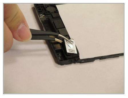
• Using the tweezer, pull out the speaker located on the inside of the back cover of the phone.
