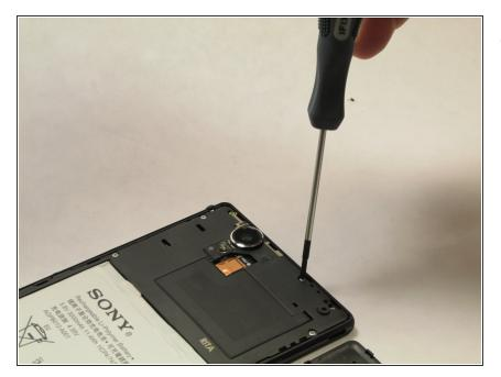
Using the Phillips #00 Precision screwdriver, take out 8 silver screws (3.15mm) and 5 gold screws
