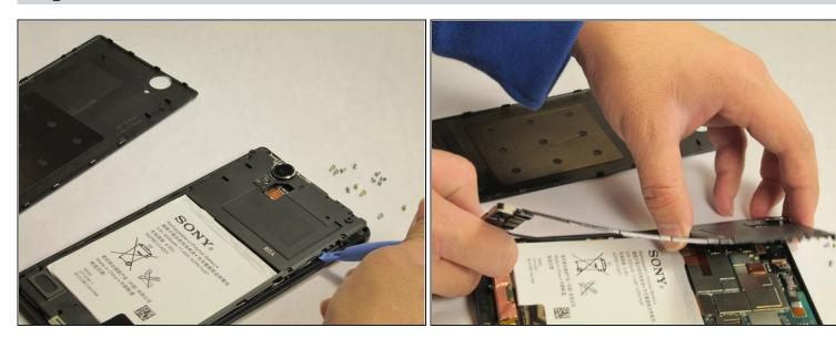
• To remove the internal cover, use the plastic spudger tool and pry the cover from the phone as shown in the picture.
