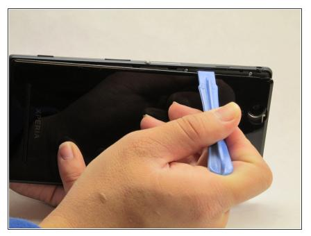
Using the spudger, pry open the back cover by starting alongside the edge of the back cover.
