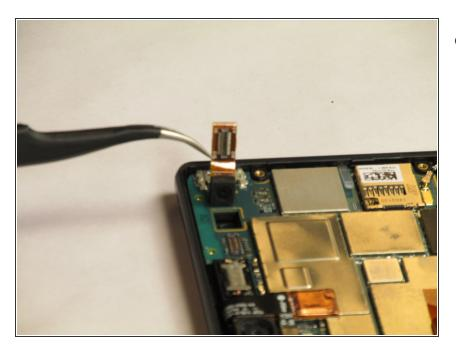
Using the tweezer, carefully pry open the chip for the front facing camera as shown. Then using the tweezer, carefully remove the front facing camera component.
