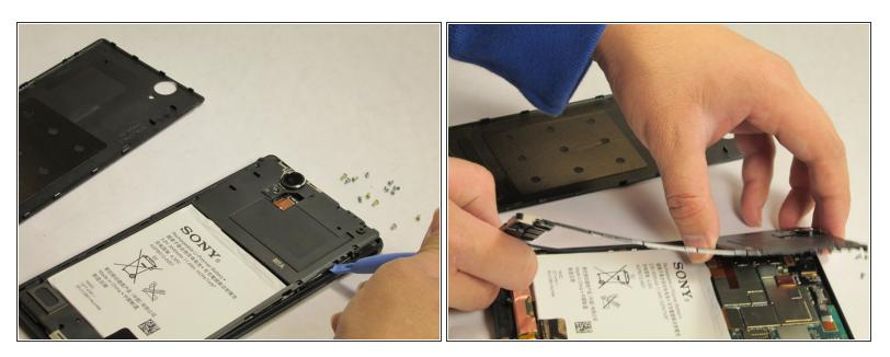
• To remove the internal cover, use the plastic spudger tool and pry the cover from the phone as shown in the picture.
