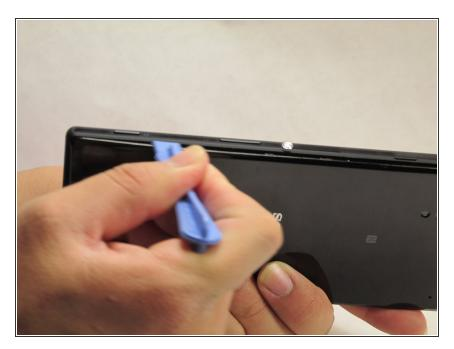
Once the part of the back cover has been opened up. Slide the spudger to pry completely detach the cover from the phone.
