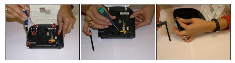
• Remove all 1/4 inch screws(6 total) with a (+PH00) screwdriver. Open slowly not to damage the display data cable.
