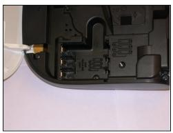
• Turn the device to it's side toward the bottom of the keyboard. Then pop open the case and remove the batteries.
