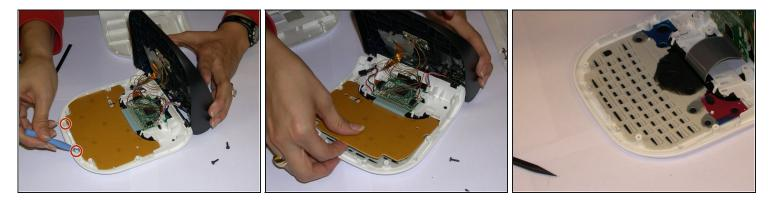
• Use a plastic opening tool to remove the flat-panel membrane keyboard. Lift up and set aside.
