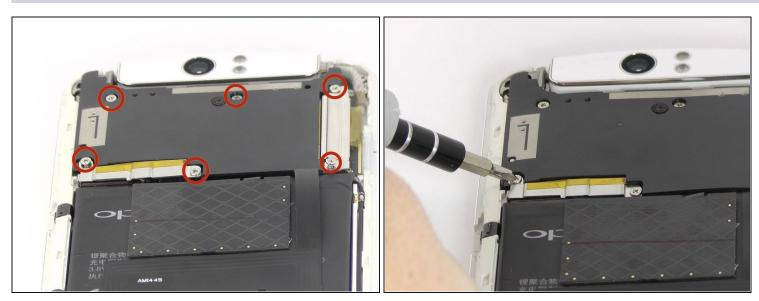
• Remove the six 4mm long screws holding the motherboard in with the ph0 Phillips head screw driver.
