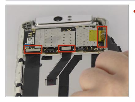
• Use <u>tweezers</u> or fingers to remove the three connector tabs.
