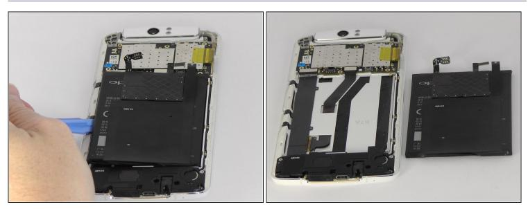
• Use the blue opening tool to carefully pry the battery from the sticky tape that attaches it to the device.
