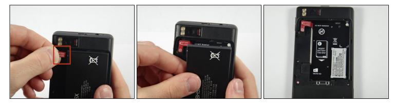
• Pull up on the red battery release tab and pull the battery out of the phone.
