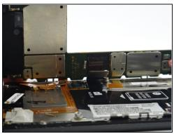
• Use a spudger to disconnect the cable connector.
