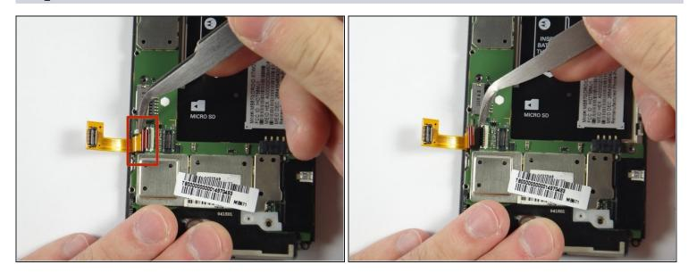
• Using tweezers, carefully disconnect the cable connector by pulling the cable out.
