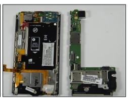
• Using a spudger, remove the camera. Lift up the motherboard and slide the spudger under the camera.
