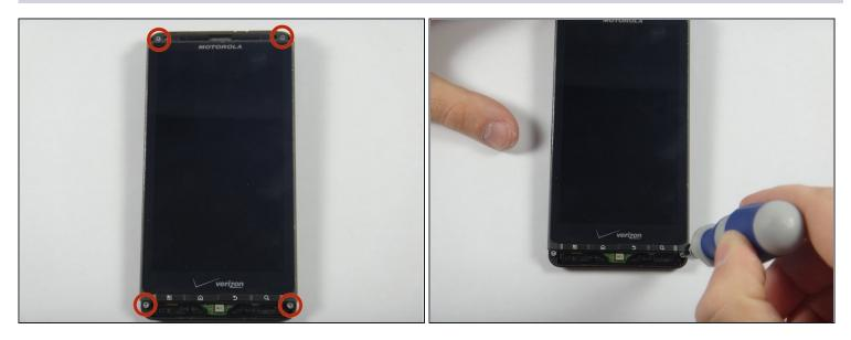
• Remove the circled screws using a T-5 torques.. These screws should be 5.8 millimeters in length.
