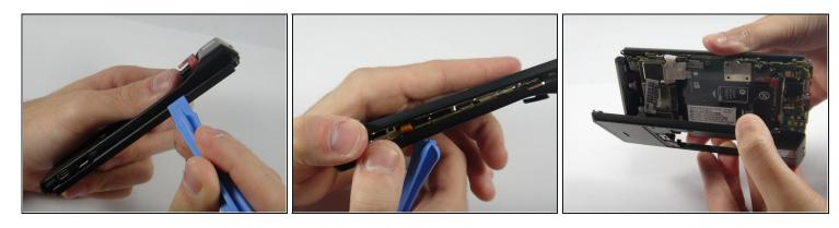
• Using a plastic opening tool, snap open the phone. It should separate into a front piece with the hardware and a plastic backing.
