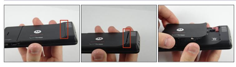
Slide the plastic case off of the back of the phone, exposing the battery.
