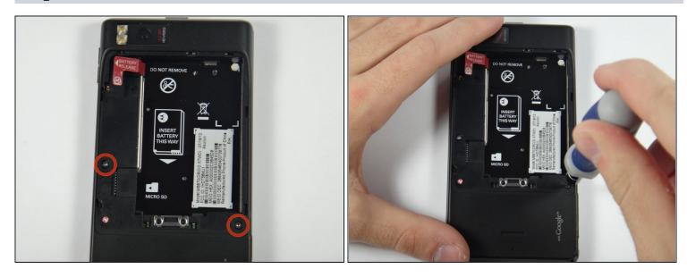
• Remove the circled screws using a T-5 torques. These screws will be 4.3 millimeters in length.
