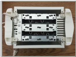
Using a Phillips #1 screwdriver, remove the four screws on the underside of the toaster.
