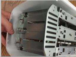
After removing the side casing, you will locate two white tabs. Using a needle nose pliers lift these tabs so they stick up instead of laying flat.
