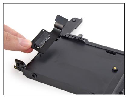
Remove the PCIe SSD cable from the drive tray.
