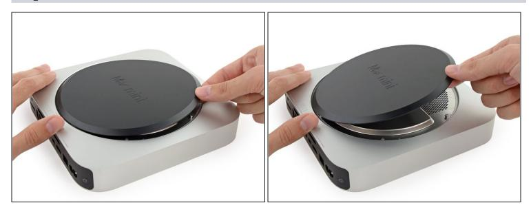
• Lift and remove the bottom cover.
