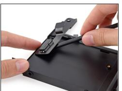
Slip the flat end of a spudger under the SSD cable to lift it off the adhesive holding it to the drive tray.
