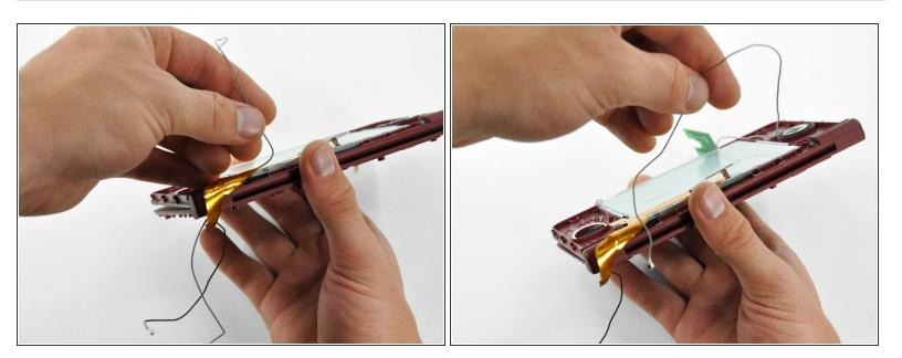
Pull the Wi-Fi antenna cable through the right hinge connecting the front bezel and upper case.
