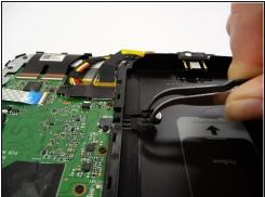
• With <u>tweezers</u> gently squeeze and remove docking indicator device
