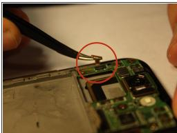
Disconnect all wires and bands from microphone, SIM card port and side bottons
