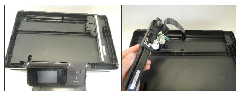
• Gently pick up the scanner piece as shown to see the bottom side and wiring.
