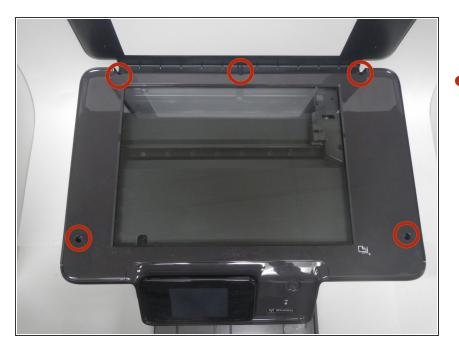
Using the T9 Torx Security screwdriver bit, unscrew the five 12mm screws shown.
