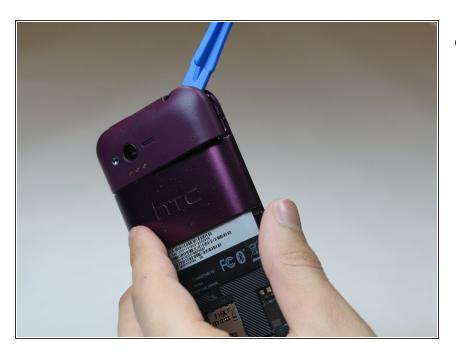
Remove the top back casing of the phone.
