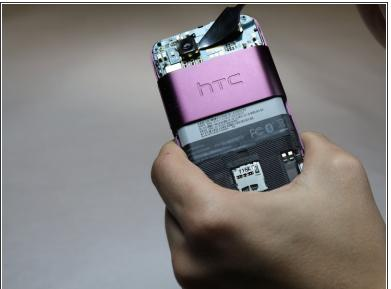
Pry the camera off of the board and replace it with your new camera.
