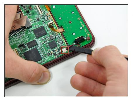
Using the flat end of the spudger, pry the battery cable up off its socket on the motherboard.
