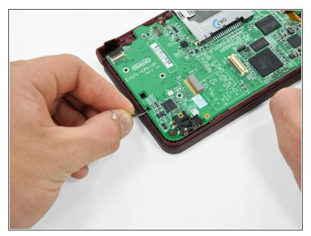
• Deroute the microphone and antenna cables through the slot in the motherboard.
