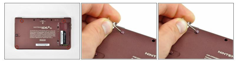
• Remove the four rubber screw covers on the lower case by prying them up with a push pin.
