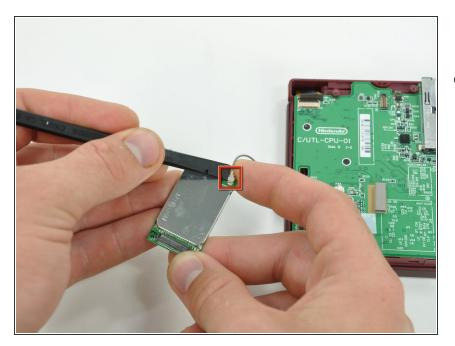
Use a spudger to pry the Wi-Fi cable off its socket on the underside of the Wi-Fi board.
