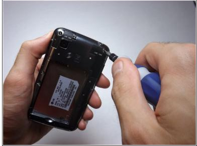
Use the PH #000 screwdriver to remove the six screws from the midframe
