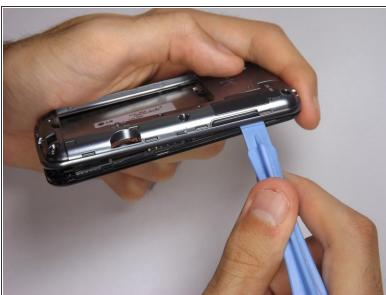
Using the plastic opening tool, work gently to go around the perimeter of the phone and remove the midframe.
