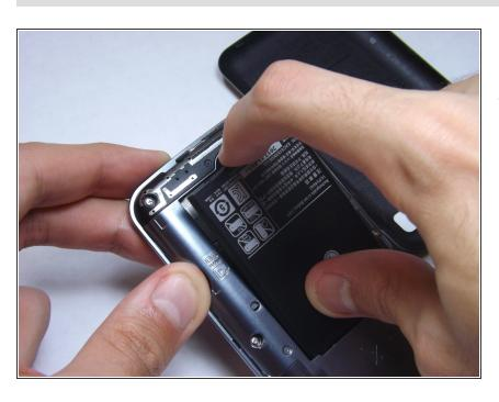
Lift the battery out of the phone and replace with your new one.
