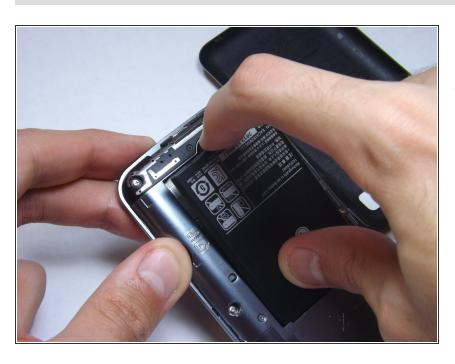
Lift the battery out of the phone and replace with your new one. To reassemble your device, follow these instructions in reverse order.
