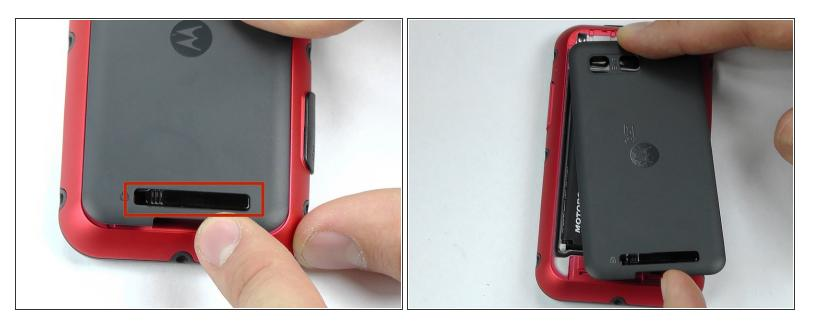
Remove the back cover of the phone by sliding the bottom black button to the unlock position and lifting it up.
