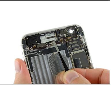
Grasp the antenna connector with a pair of tweezers and gently lift it from its retaining clip on the logic board.
