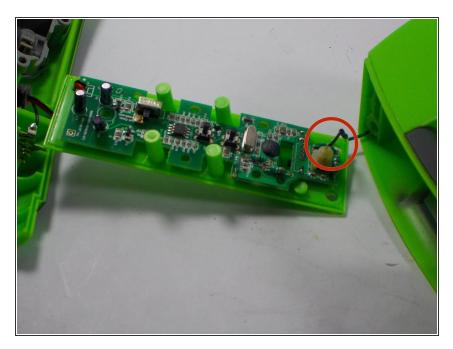
• Disconnect circuit board from power leads, and install new circuit board.
