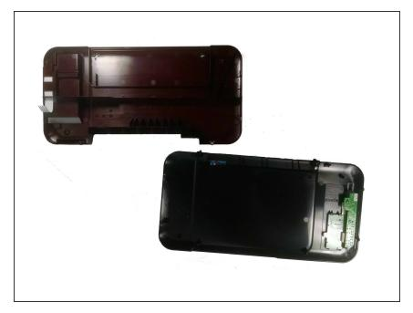
You will need to remove the button, button circuit board, and screen in order to replace the control panel.
