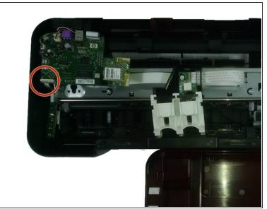
• Once the top is loose, there will still be a connection wire between the printer and the cover. This wire will be about one inch wide and white, located under the buttons.
