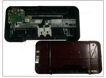
Now that the top cover is removed from the printer body you will need to separate the control panel from the maroon panel.
