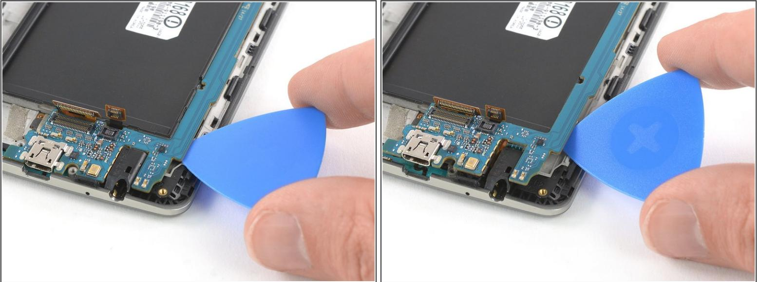
**⚠** During these next few steps, make sure to avoid damaging the flex cables you disconnected.
