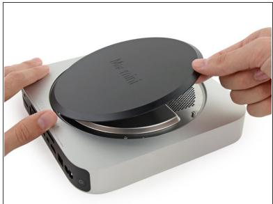
Lift and remove the bottom cover.
