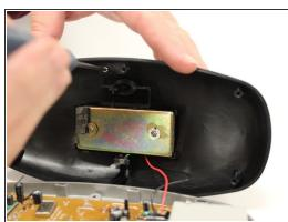
Inside the base cover, locate the screw holding the antenna in place and use a Philips #00 screwdriver to remove the 6mm screw.
