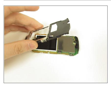
Gently remove the plastic and metal framework of the phone by lifting it up.
