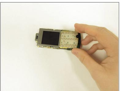
The circuit board for the buttons is now free to be removed and replaced.
